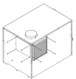
Figure 4 – Metal Panel Covering Side Combustion Air Inlet
